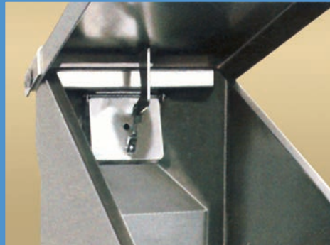
Optional dust collection units can be added to the tops of the bins to effectively control dust as bins are being filled.
