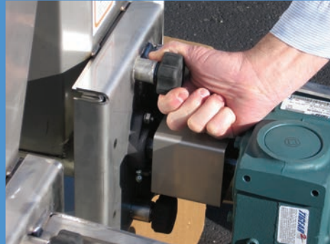
Unscrew the two mounting bolts.
