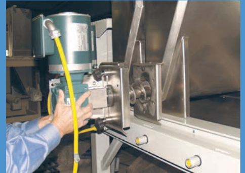
Remove the motor drive from the micro bin.
